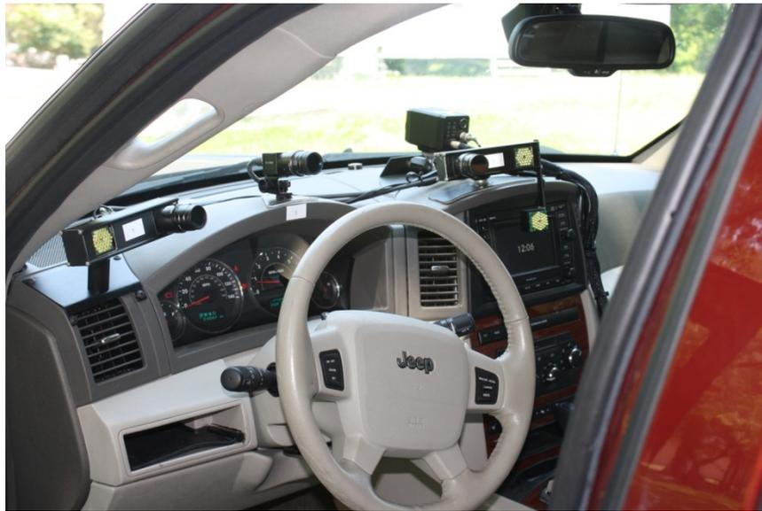
**Figure 1. Eye tracking system camera placement.**
