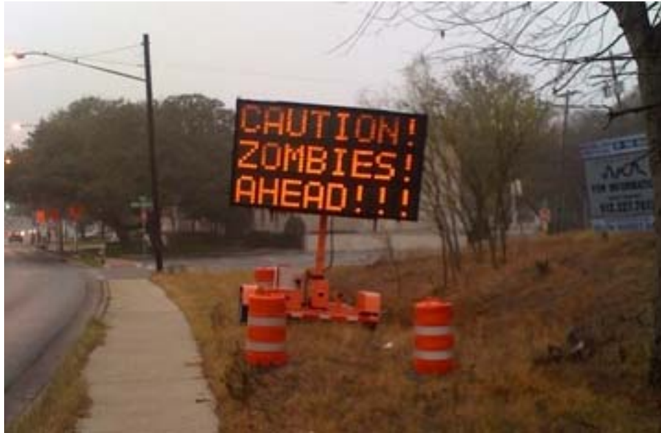
Figure 15. A portable changeable message sign (PCMS) that was “hacked.”
