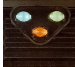
RGB LED Pixel used in OOH Media
